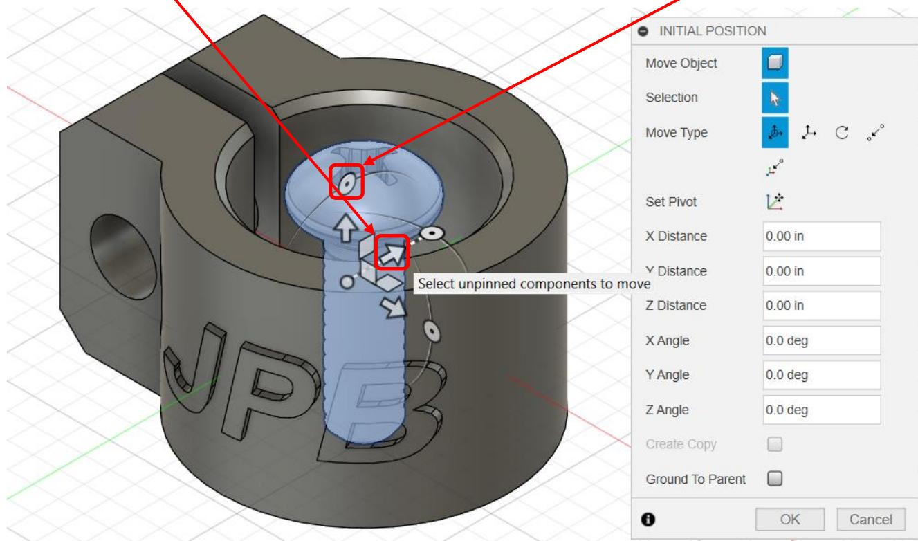
The screw position is not critical. The **underside of the screw head** just needs to be visible.
