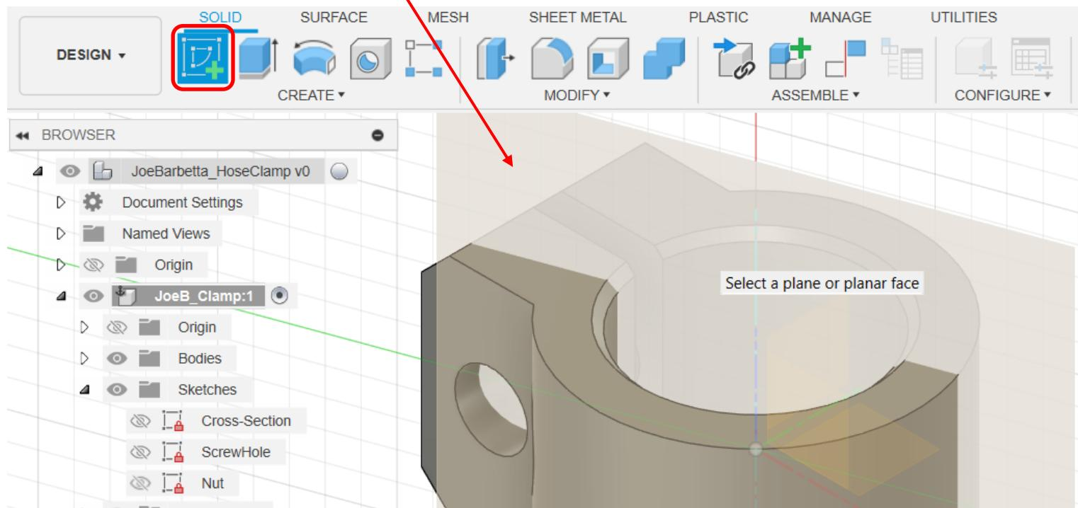
If the Sketch view is rotated, as shown below, it should be rotated so the Z-axis is straight up. Normally, 2 curved arrows will appear at the View Cube when the mouse hovers over it. However, because the Sketch was created on a angled Construction Plane, these arrows are not available.
